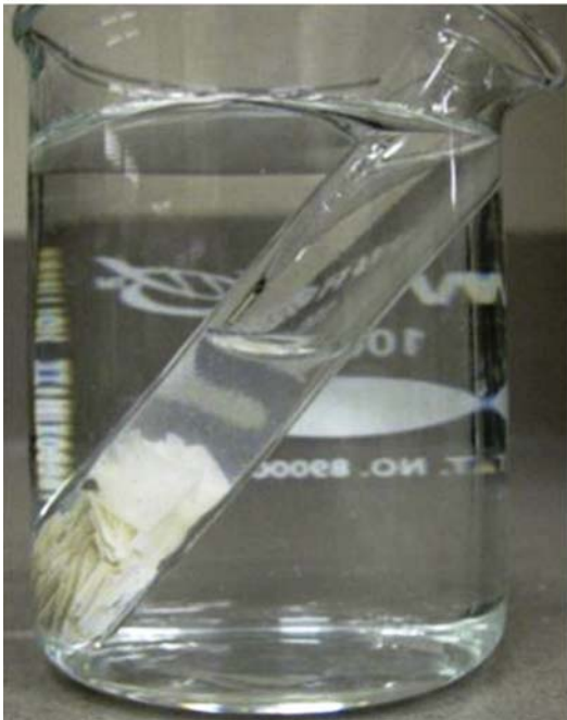
FIGURE 3.23 Color change from white (A) to red-violet (dark gray in print versions; B) during Fujiwara test indicating membrane exposure to halogens.
