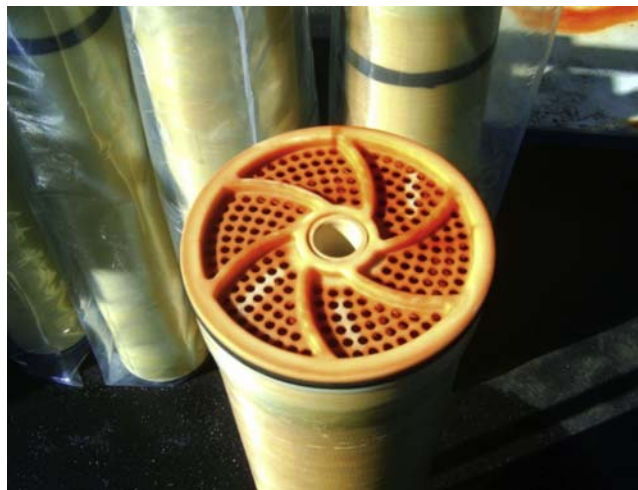
FIGURE 6.5 Coagulant residue on the reverse osmosis membrane feed due to iron coagulant overdosing.
