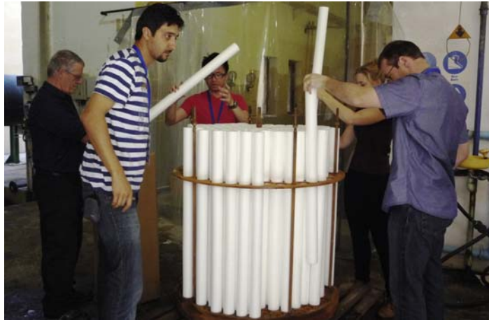
FIGURE 5.12 Cartridge filter loading.
