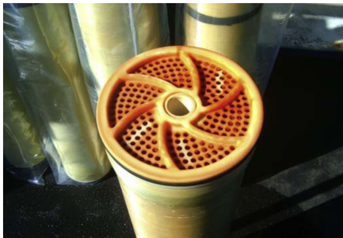
FIGURE 3.12 Reddish/brown discoloration of RO elements caused by overdosing of ferric coagulant.
