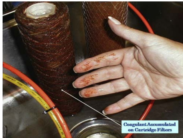
FIGURE 6.4 Coagulant accumulation on cartridge filters due to iron coagulant overdosing.
