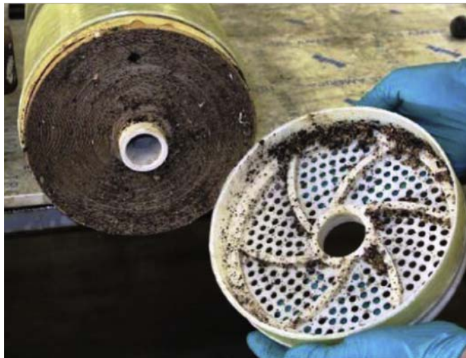
FIGURE 3.15 Accumulation of particulate debris on the front of the element and end cap.
