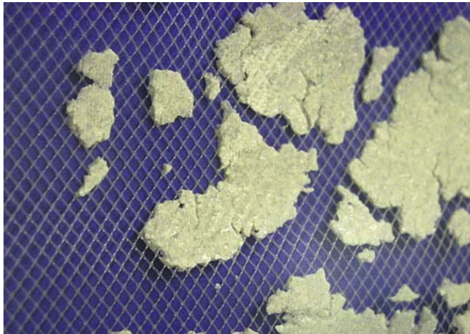
FIGURE 3.5 Accumulation of scale on the membrane brine spacer.
