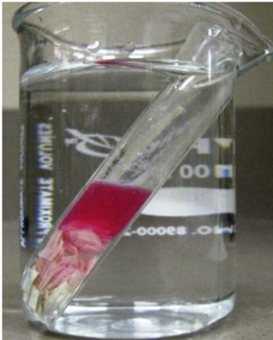
FIGURE 3.23 Color change from white (A) to red-violet (dark gray in print versions; B) during Fujiwara test indicating membrane exposure to halogens.
