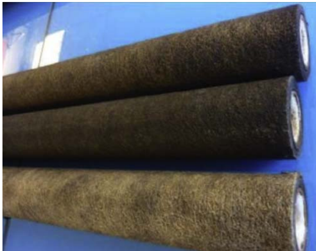
FIGURE 6.3 Cartridge filters with dark brown/black discoloration as a result of the use of poor quality ferric chloride.
