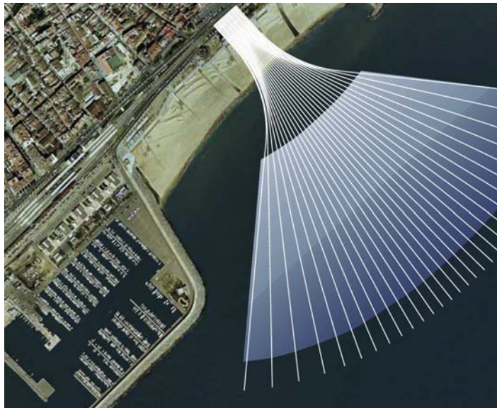
FIGURE 4.5 HDD Intake of San Pedro del Pinatar SWRO plant, Spain.
